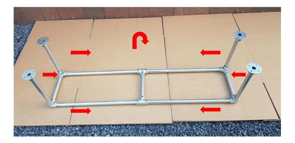
Lay the frame on its back and pull legs inward slightly, tighten all set-screws in the cross member.
