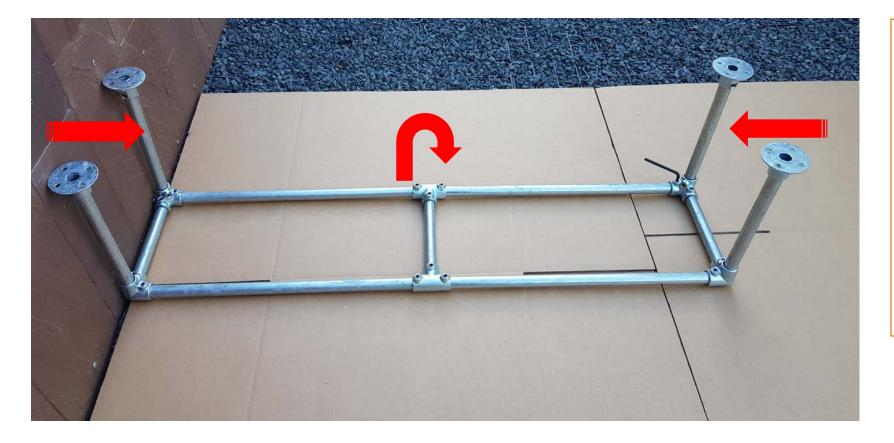
Tighten your set- screws as firmly as possible as this ensures minimal sag in your bars. Pulling in the frame legs while you do so also helps.
