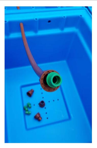
Soaking the end of the lines in warm/hot water helps with this process.
